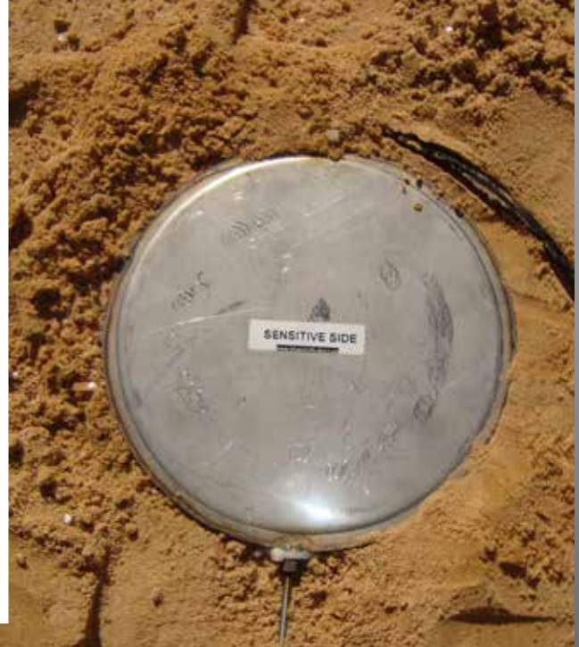
Electronic pressure monitors were placed beneath the restructured embankments to measure settlement. Photo: Ed Bell Construction
