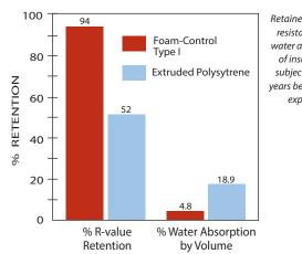
resistance and water absorption of insulations subjected to 15 years below grade exposure
